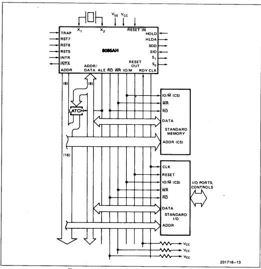
Figure 9. 8085 System (Using Standard Memories)
