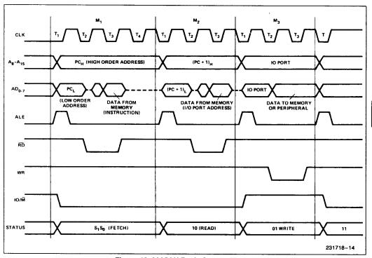
Figure 10. 8085AH Basic System Timing
