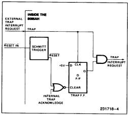
Figure 4. TRAP and RESET In Circuit
