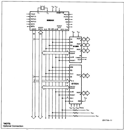
Figure 7. 8085AH Minimum System (Standard I/O Technique)
