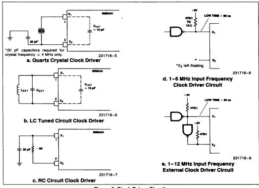
Figure 5. Clock Driver Circuits
