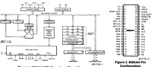
Figure 1. 8085AH CPU Functional Block Diagram
