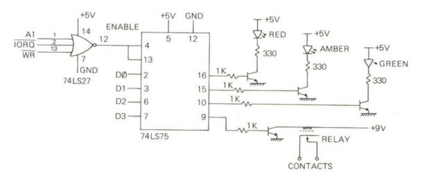
The signals to this circuitry (A1, IORQ and so on) need to be connected to the computer through an *edge connector*, a connector that clips over the back edge of the circuit board. Here is the arrangement of the signals on the computer.
