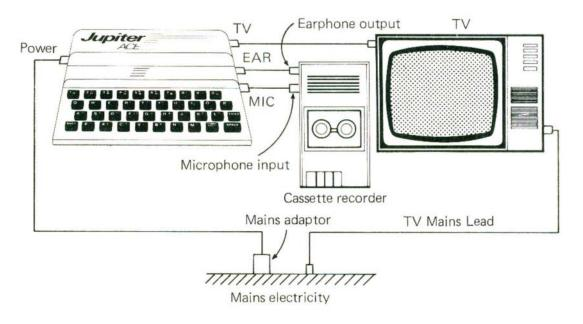
A tape can have several programs, coded by the computer into a signal suitable for recording on tape. Each program has a name of up to ten characters, again coded electronically onto the tape. Let us suppose that your tape has an interesting program
