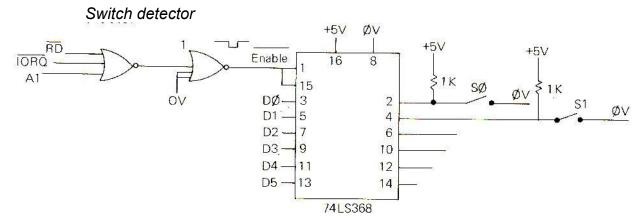
Switches S2 to S5 are similar to SO and S1, each with a 1K resistor, and are connected to pins 6, 10, 12 and 14.
