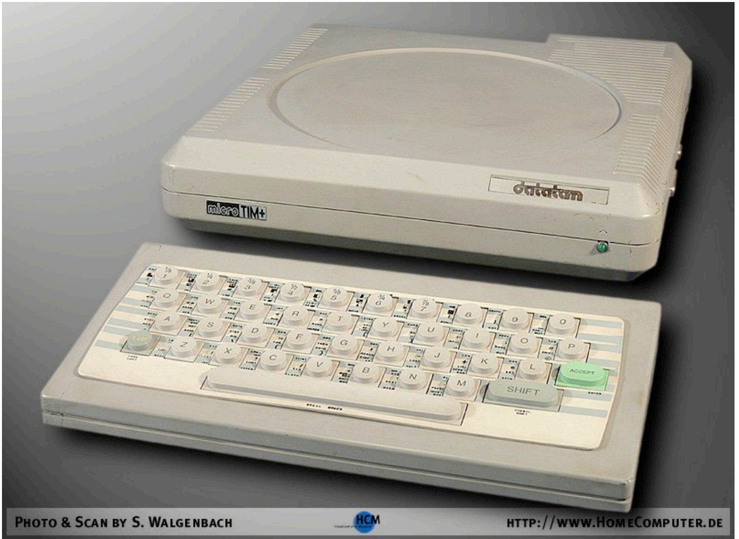
IPTVT MicroTim+ (it has 80Kb of RAM but it still comes from 48Kb series)
