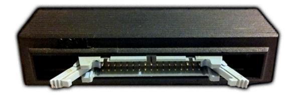
This is the front part of the interface which connects into the QL expansion slot
