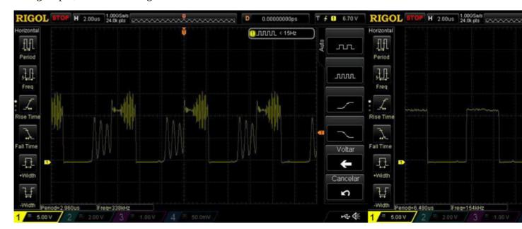
The Spectrum Next noise before and after the capacitor mod
