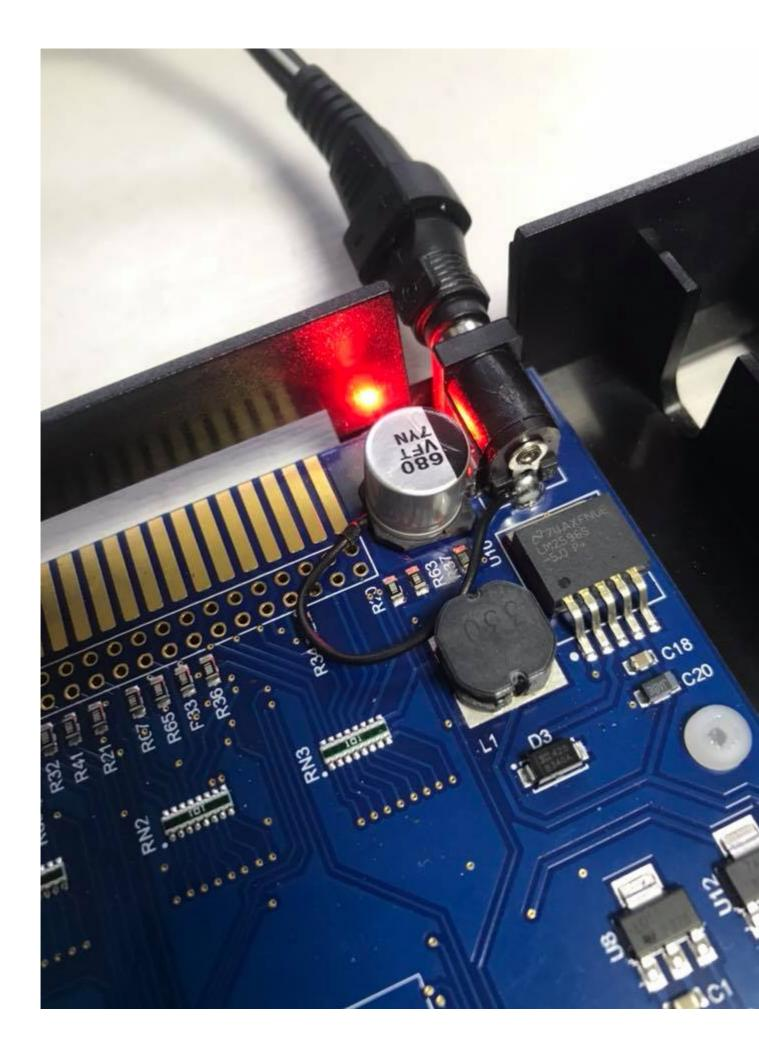
The capacitor soldered to the 9V connector. The black notch indicates (-) polarity, thus soldered to the side of the connector, while the (+) leg of the capacitor goes in the middle of the connector. Photo by Jon Gratton (FB Next group).
