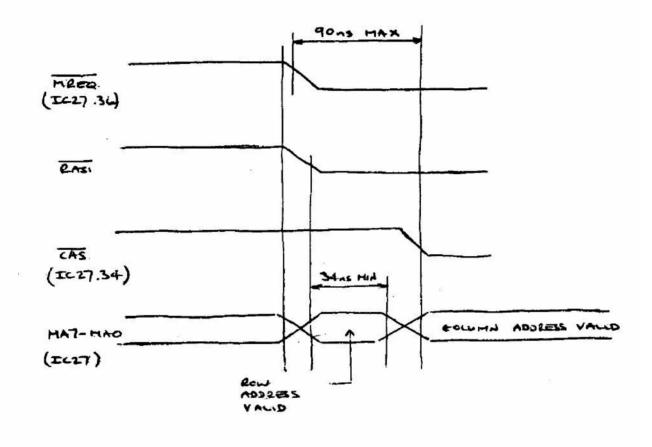
FIGURE 1.2 UNCONTENDED RAM RAS/CAS TIMING (READ CYCLE SHOWN)
