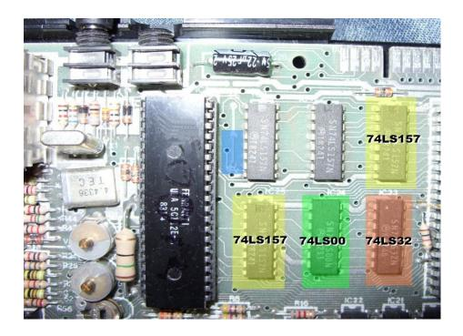
Issue 3 PCB - Jumper positions highlighted in blue (shown with heatsink removed)
