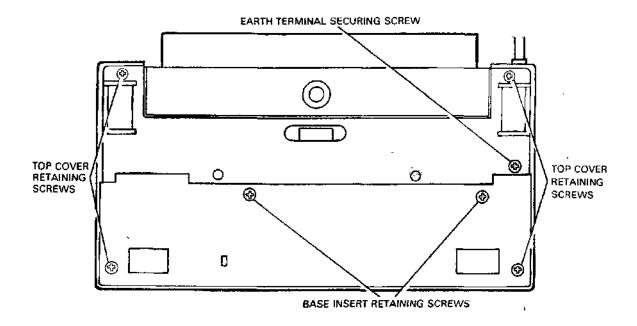
FIGURE 3 TOP COVER & BASE INSERT ATTACHMENT POINTS
