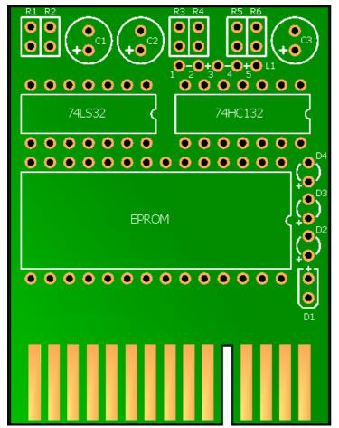
R1, R2 and C1 control the A15 line. R3, R4 and C2 control the ROMCS line.
